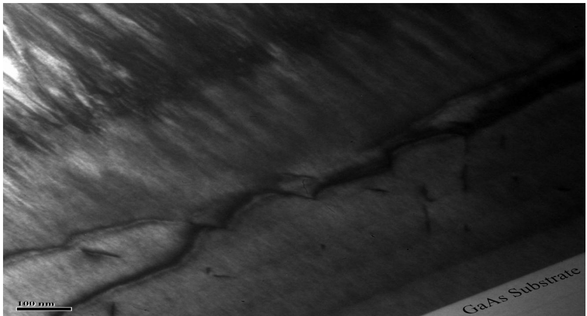
Fig 5-2: Cross-sectional bright field TEM image of linearly-graded quaternary alloy grown at 500°C.
