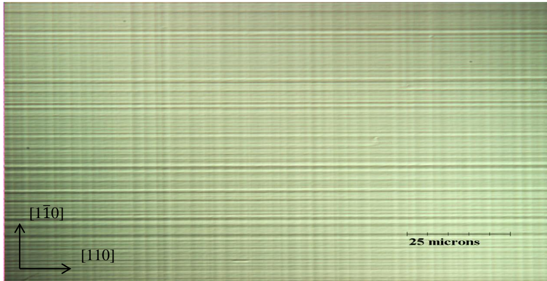
Fig 4-2: Optical microscope image of cross-hatch in \text{In}_{0.3}\text{Ga}_{0.7}\text{As} layer grown metamorphically on GaAs (001) substrate.
