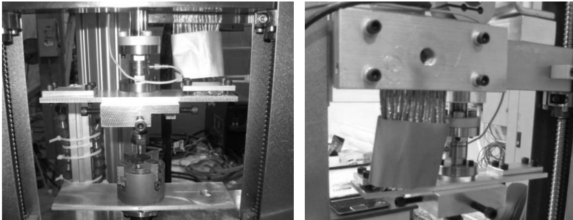
Figure 11: Second design concept for attaching upper welding cable to tribometer
