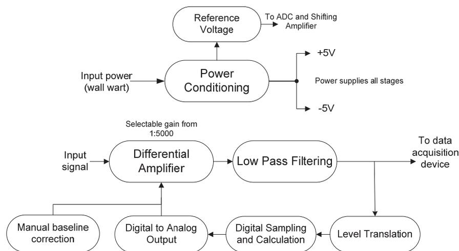
**Figure 2-4** Block diagram of the force amplifier design. The output from the low pass filter block is level translated and sampled for use in automatic baseline correction.
