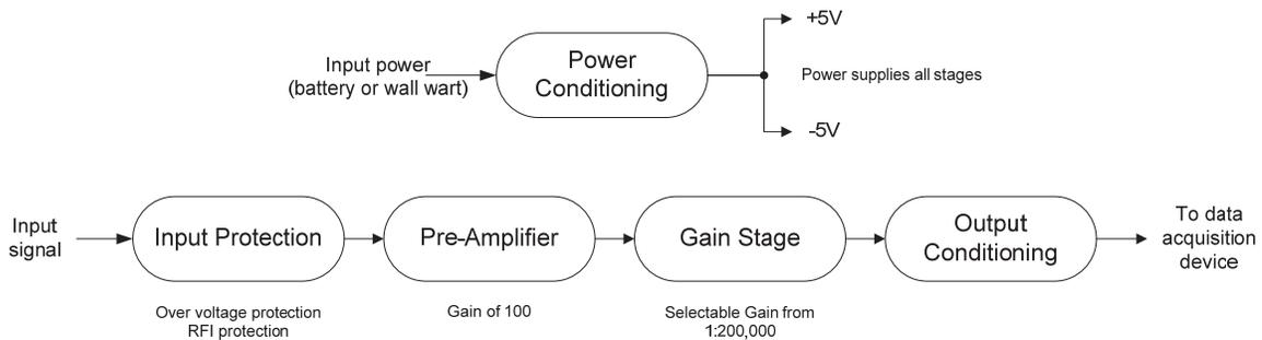
**Figure 2-1** A block diagram of the EMG amplifier design. The power conditioning block supplies power to all operational amplifiers in the pre-amplifier and gain stage blocks.
