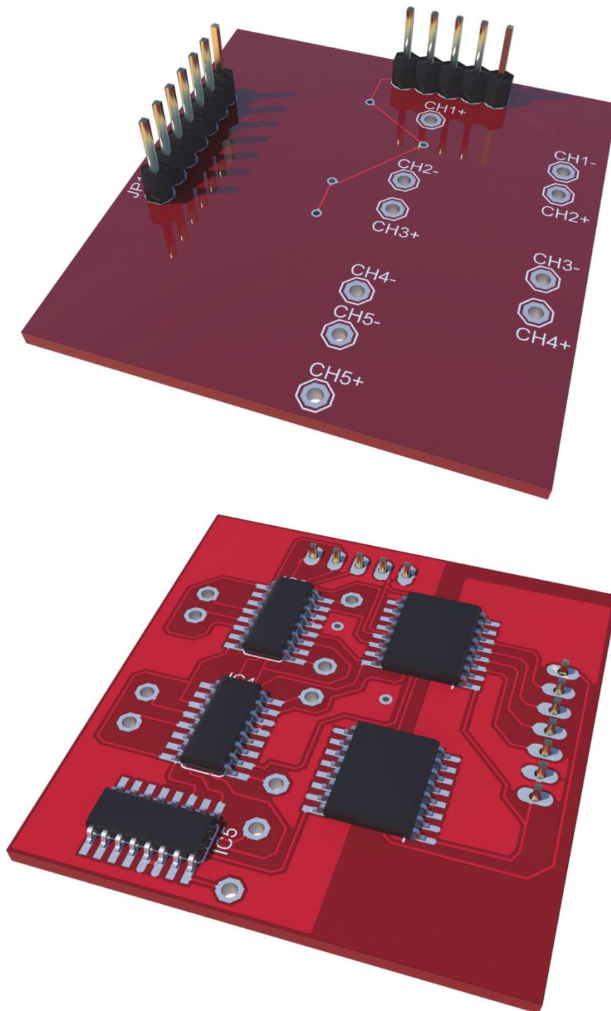
**Figure 2-10** Printed circuit board 3D renderings of the 5 channel breakout box.
