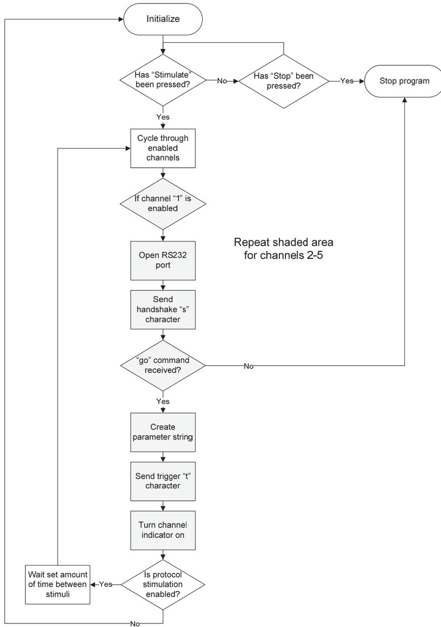
**Figure 2-11** Software flow chart for the LabVIEW program that controls the hardware stimulator.
