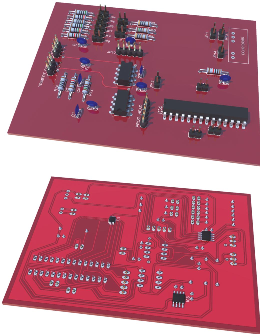
**Figure 2-6** Printed circuit board 3D renderings of the amplifier. The top of the board is shown above and the underside of the board is shown below.
