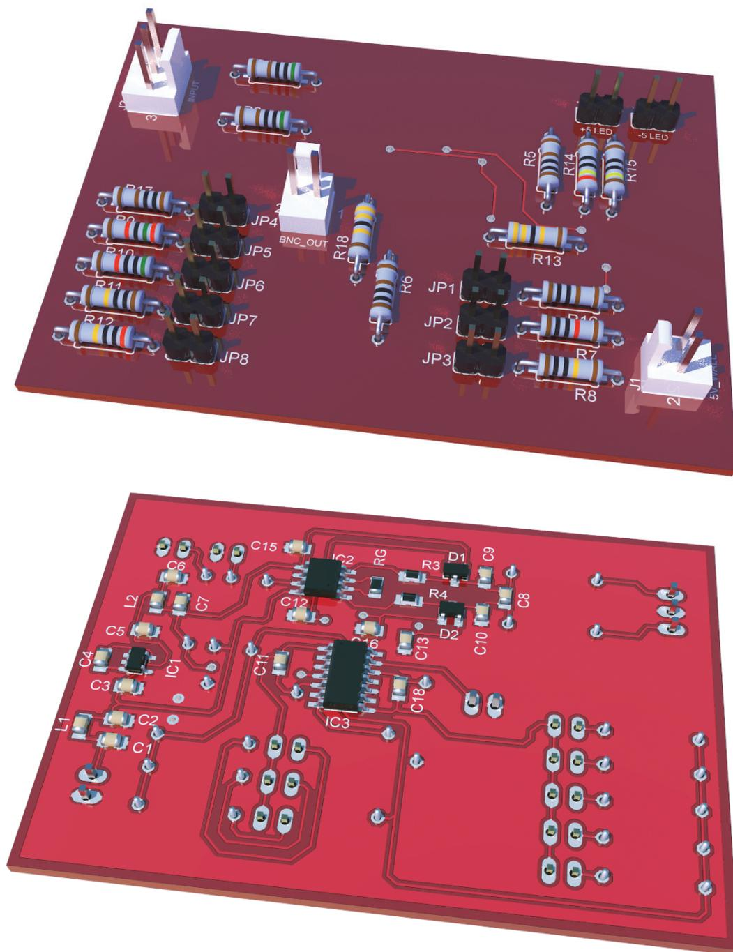
**Figure 2-3** Printed circuit board 3D renderings of the amplifier. The top of the board is shown above and the underside of the board is shown below.
