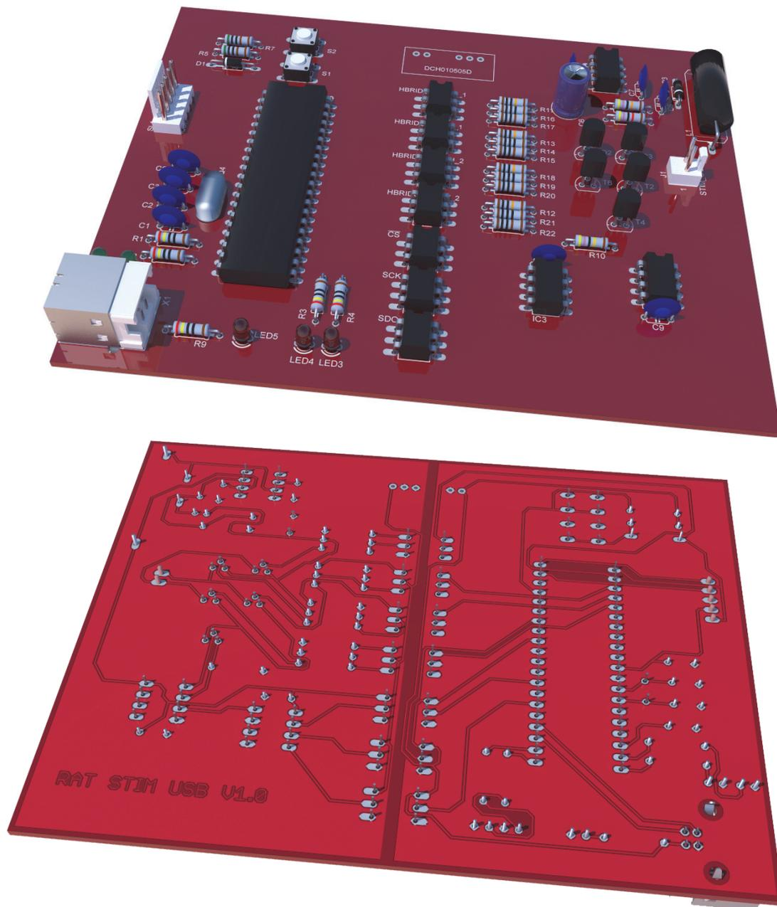
**Figure 2-9** Printed circuit board 3D renderings of the muscle stimulator. The top of the board is shown above and the bottom of the board is shown below.
