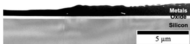
FIGURE 4 Bright-field TEM image of a cross-section of the multiple-layer sample irradiated by a single \lambda = 400 nm, \sim 0.358 \mu\text{J} ( \sim 1.06 \text{ J/cm}^2 ) pulse. Single pulse \lambda = 800 nm irradiation at \sim 5.75 \text{ J/cm}^2 and \sim 3.60 \text{ J/cm}^2 yielded qualitatively similar TEM images, with no damage visible in the crystalline silicon
