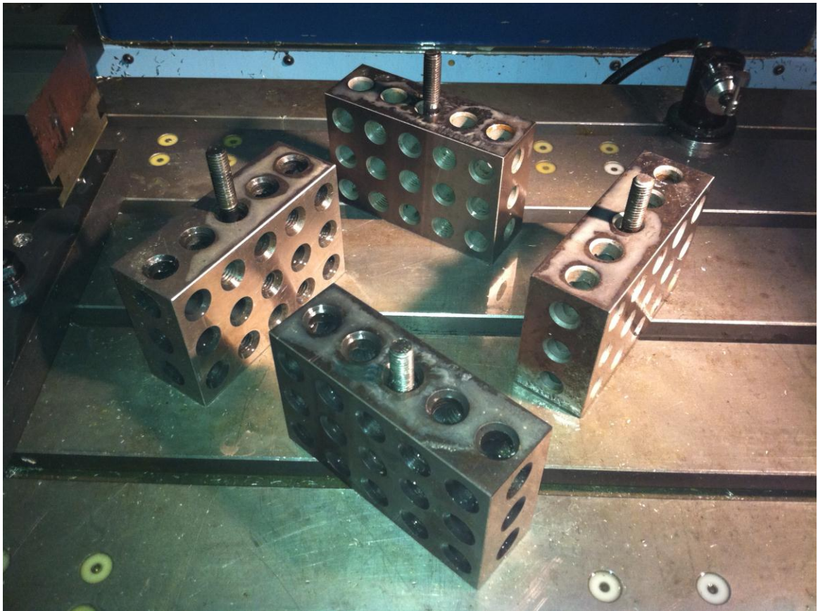
Figure 4.13. 2-4-6 blocks support of fixture for height adjustment
