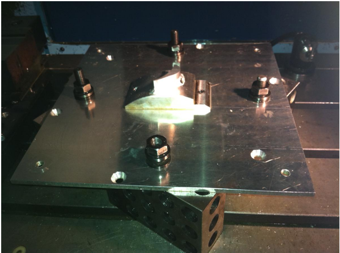
Figure 4.12. Blade loaded into the fixture which is attached to table of the Matsuura FX 5G 3-axis machine tool
