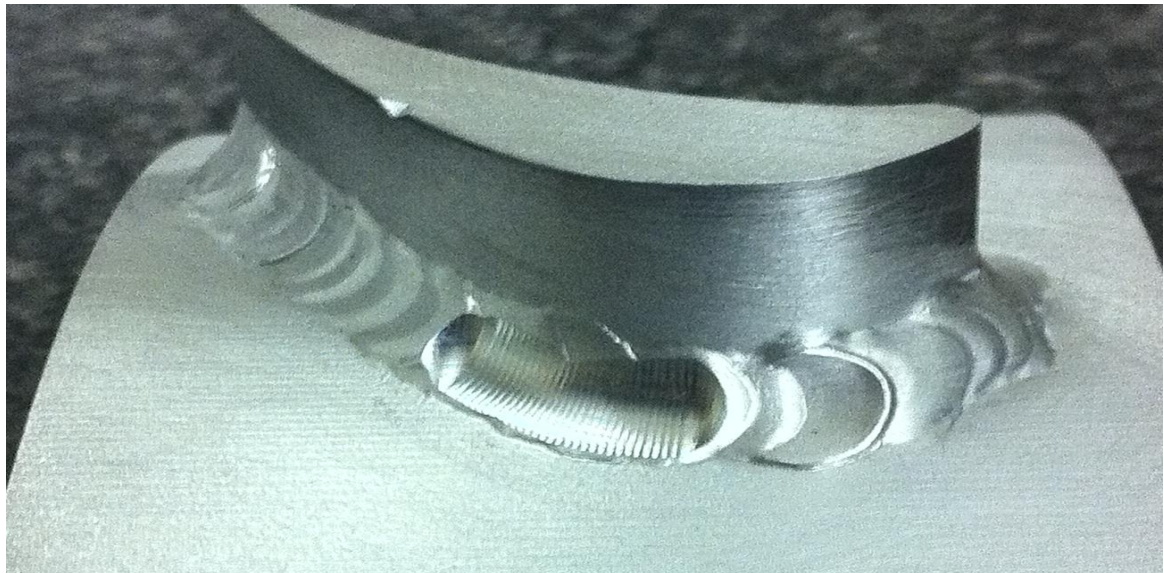
Figure 5.9 Photograph of a machined misaligned blade assembly for the case of negative 0.5 mm and 1° clockwise
