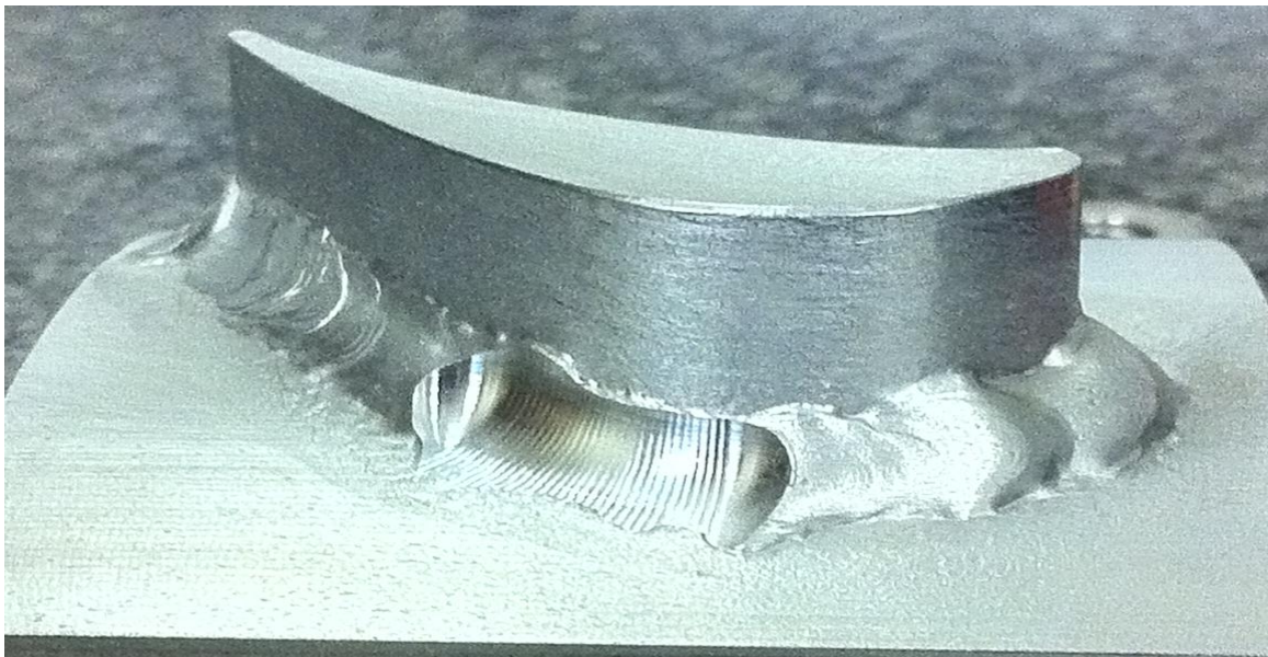
Figure 5.13. Photograph of a refurbished misaligned blade assembly for the case of positive 0.5 mm and 1° counter-clockwise
