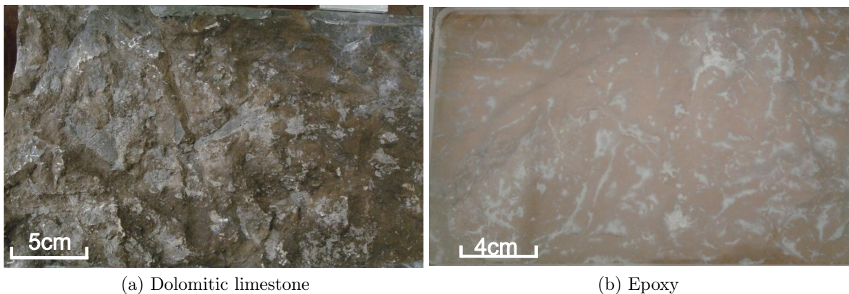
Figure 4.1: Photographs of the top view of the two types of fractures employed in these experiments.
