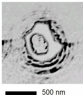
Figure 2. High magnification AFM phase image of the 5000 ms single pixel exposure from the top right corner of figure 1.
