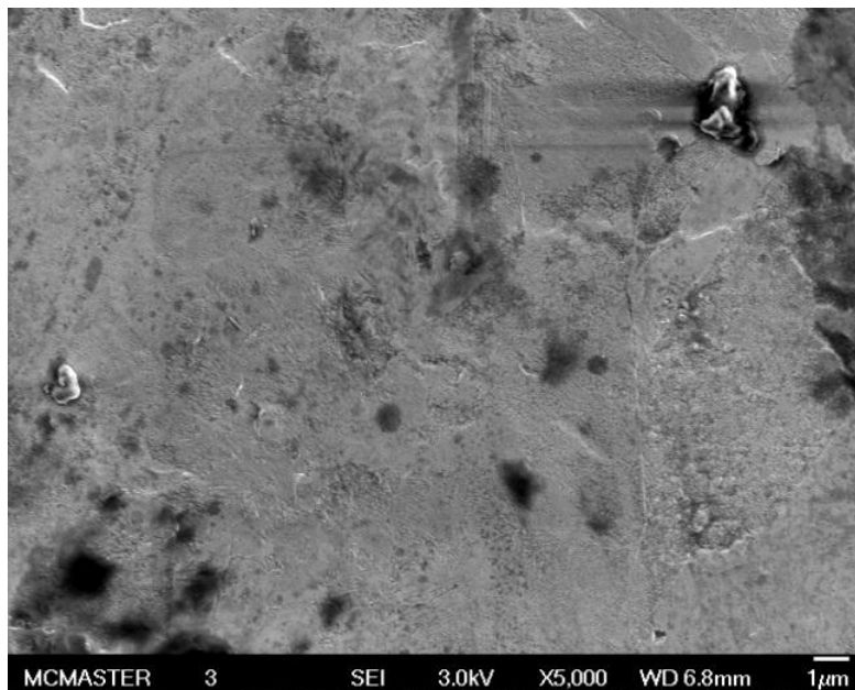
Figure 25: SEM image of planar copper sheet anodized at 40°C, in 93% H 3 PO 4 at a 6V cell voltage for 8 min in a vertical orientation
