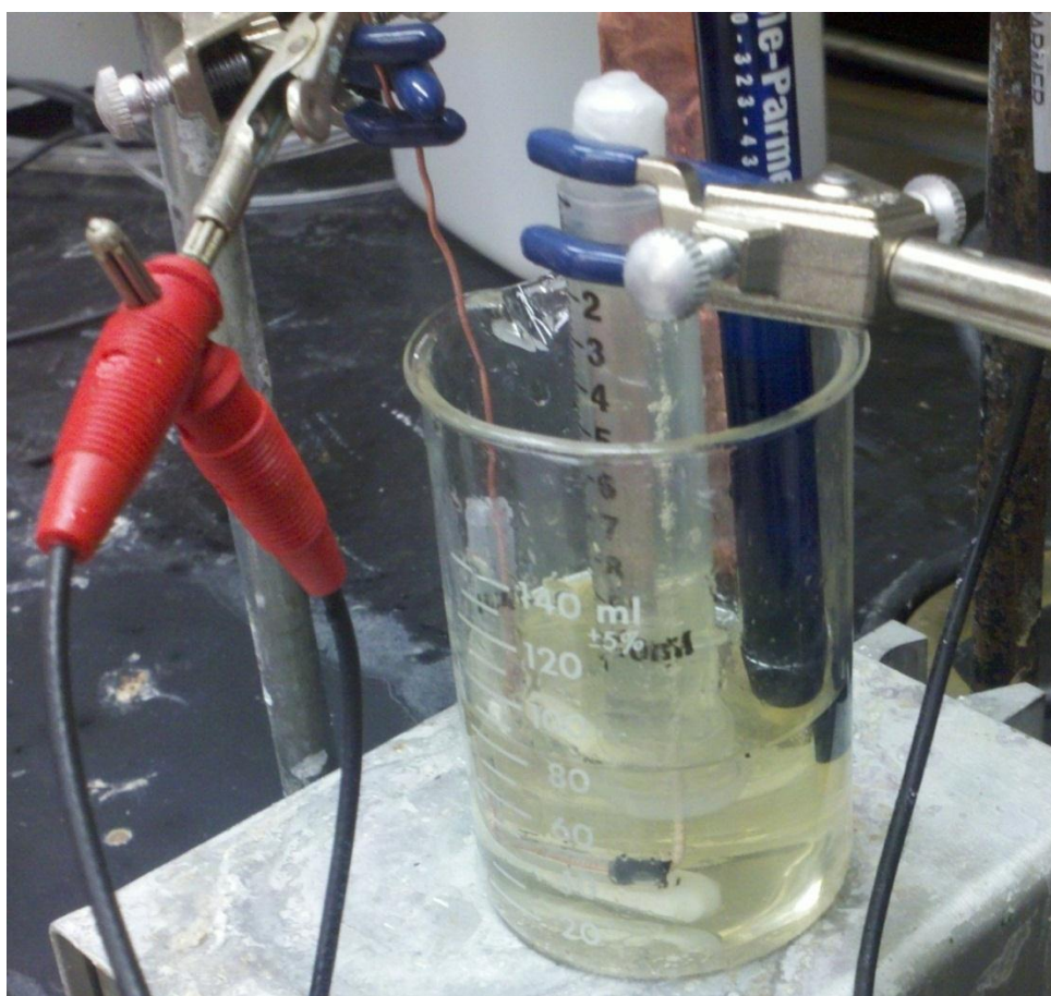
Figure 2: Experimental Setup for the Separation of Oxygen Evolution and Copper Dissolution Current Contributions
