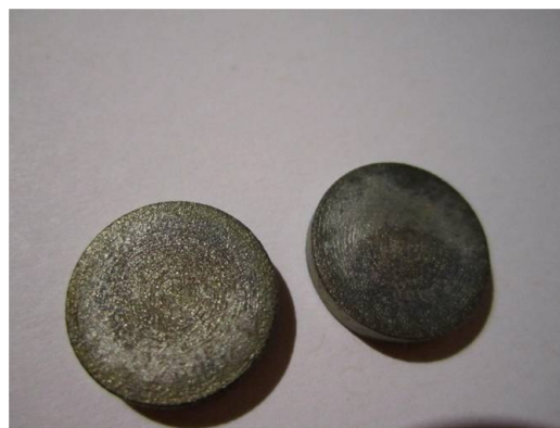
Fig. 5-47 Severe corrosion of TiC coated TZM after the corrosion test
