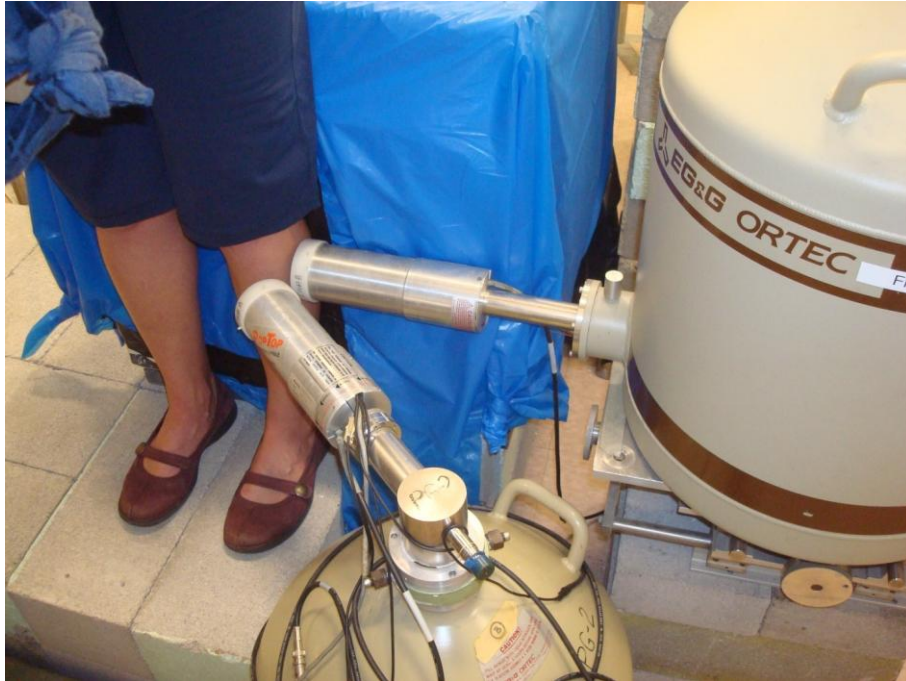
Figure 2. Photograph of a participant measurement. The participants' left leg is aligned with the collimated neutron beam, and the photons from neutron interactions in the tissue and surrounding materials are measured with two radiation detectors.
