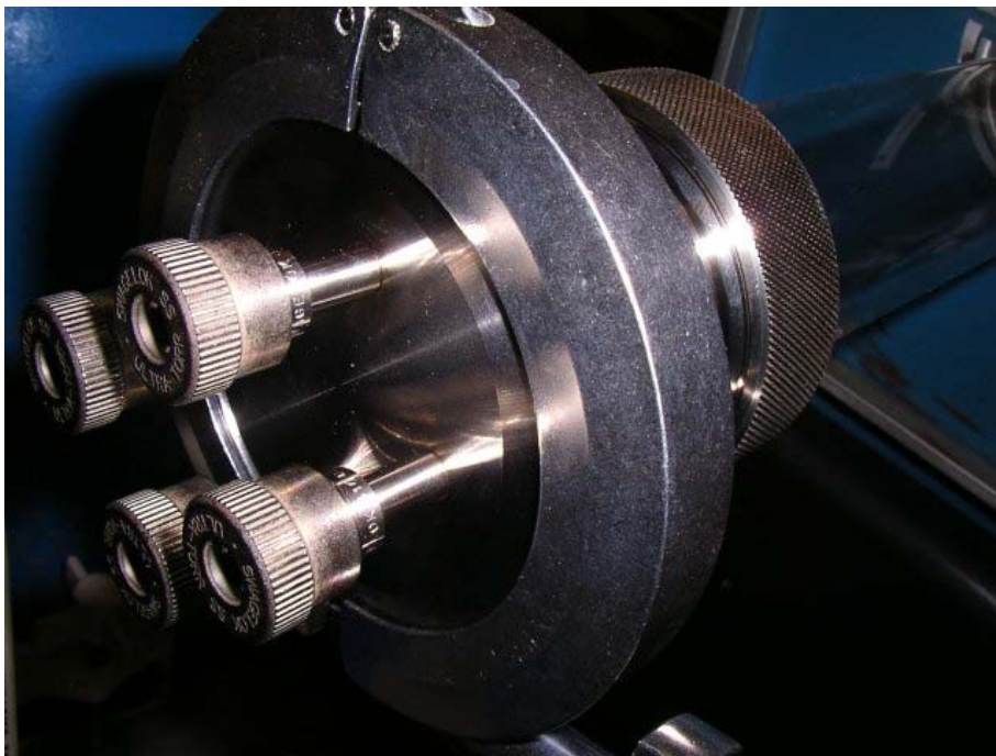
Figure4.6 Four feed-throughs for gas inlet/outlet and quartz pushing rods
