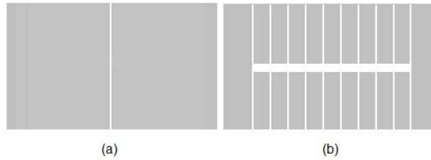
Figure 4.12 (a) Single seedline substrate; (b) multiple seedlines substrate (seedlines in white and the oxide mask in grey)
