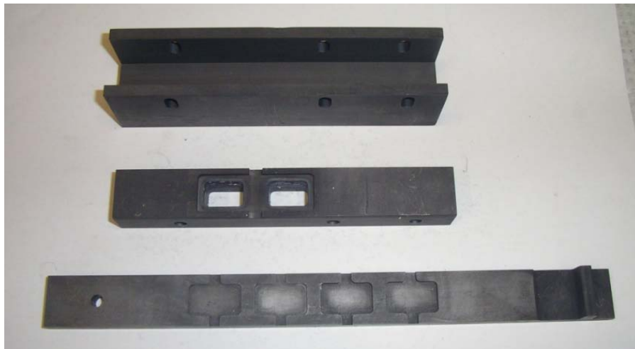
Figure4.8 Conventional LPE graphite slide boat
