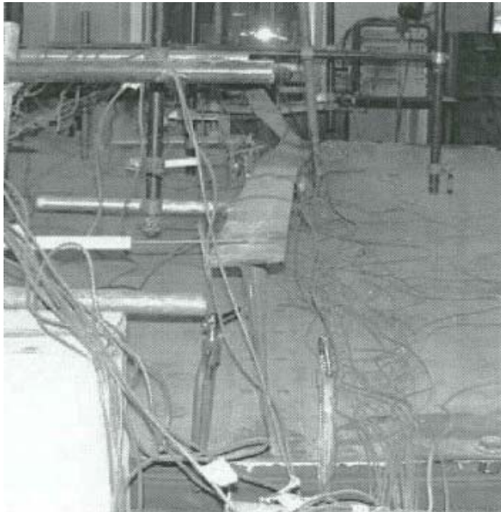
Figure 3.18 Buckling Mode of Stiffener W310X21 from Experiment
