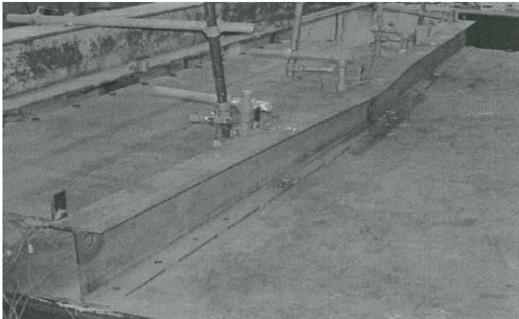
Figure 3.16 Buckling Mode of Stiffener W200X27 from Experiment
