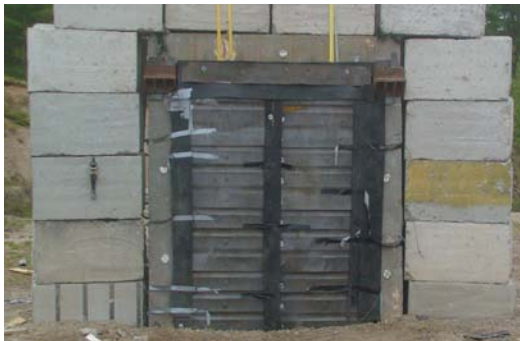
(c) Steel curtain (front view)
