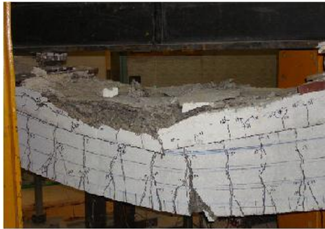
Figure 4.24: Typical concrete compression failure of control beams (Mostafa 2011)
