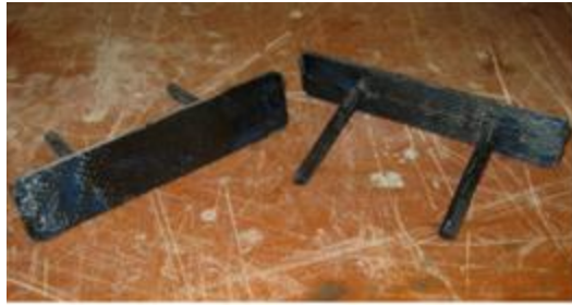
Figure 1.1: Anchors for delaying FRP debonding
