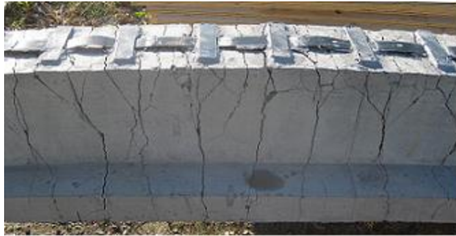
Figure 4.37: Inverted failed EBA2 specimen
