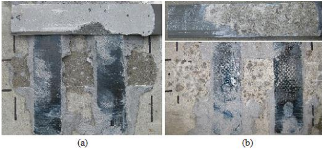
Figure 4.19: Failure plane of (a) DS8 and (b) DS9
