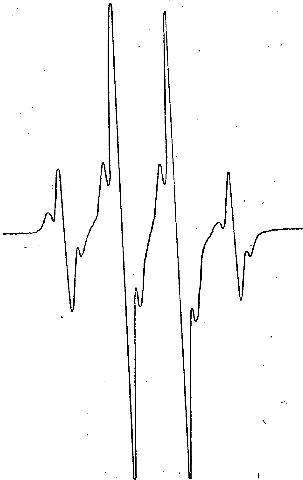
FIGURE VI-4. ESR spectrum obtained after 3 mins irradiation of 0.1 M Tl(III) acetate in 10% H 2 SO 4 at 77°K. The satellites are attributed to second order transitions.
