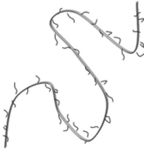
Figure 2-1: A representative cartoon depicting the presumed structure of the PCol and UV PCol scaffolds in which linear chains of amine-terminated PNIPAAm have been decorated along the backbone of type I bovine collagen, producing a comb-type grafting architecture.
