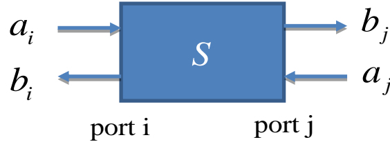
Figure 6.7 Amplitudes of in-going and out-going complex modes at two ports of a building block
