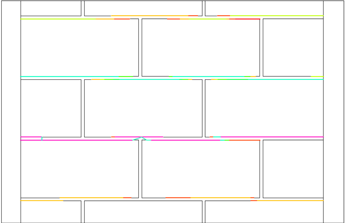
Figure B-0-8: Close-up of Crack Pattern of B-2 2.2m Wall
