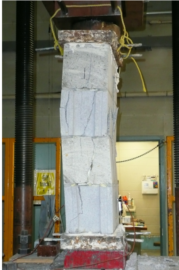
Figure 4-4: Fast Poly-mor Compression Assemblage Post Failure
