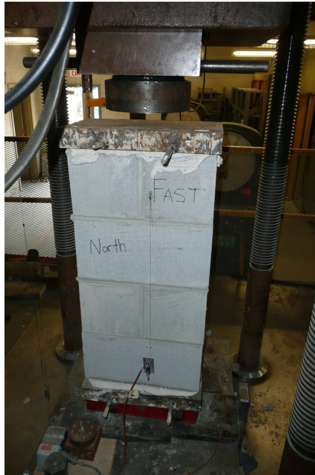
Figure 4-3: Compression Test Set-up
