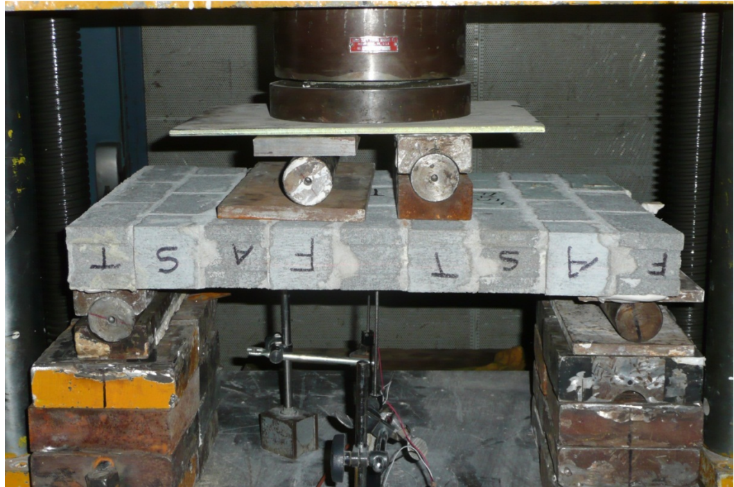
Figure 3-5: Wallette Test Set-up for Out-of-Plane Loading
