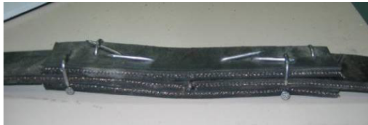
Figure 2-11: Nailed Joint (Charleson, 2009)
