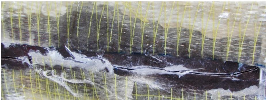
Figure 3 - 7: A close-up of the fracture induced.
