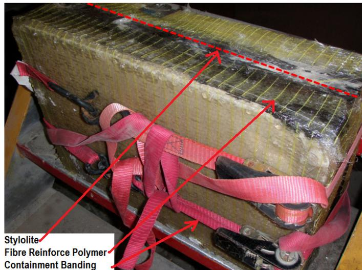
Figure 3 - 5: A sample coated in FRP and banded, prepared to undergo uniaxial loading.
