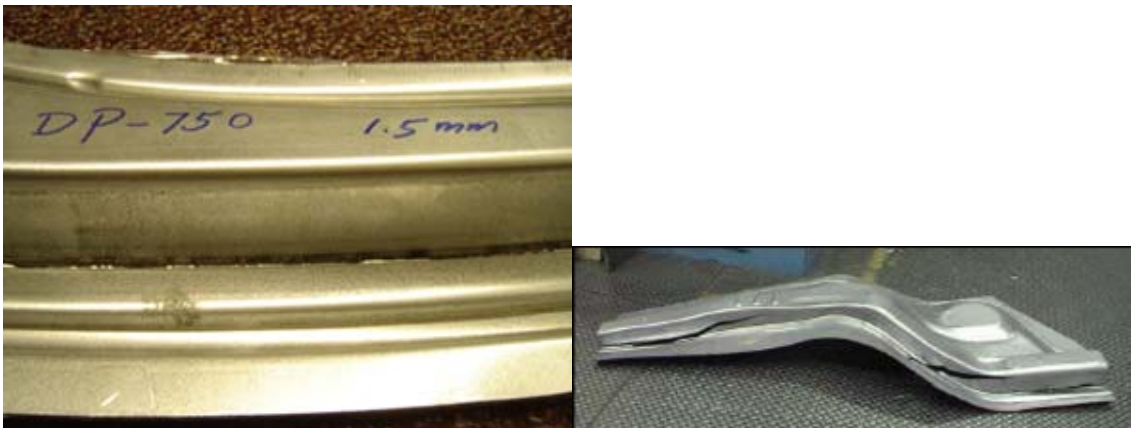
Figure 4.1. Examples of shear fracture in automotive applications.
