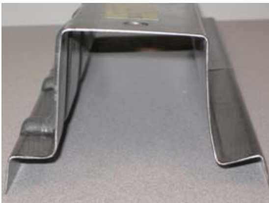
Figure 3.2. Vertical bead reduces springback
