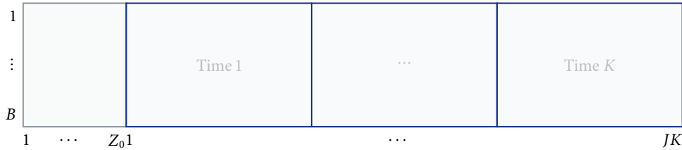
Figure 5.2: Rearrangement of the data in Figure 5.1a and Figure 5.1b to form the regressor matrix for identifying the quality model in Equation (5.2)
