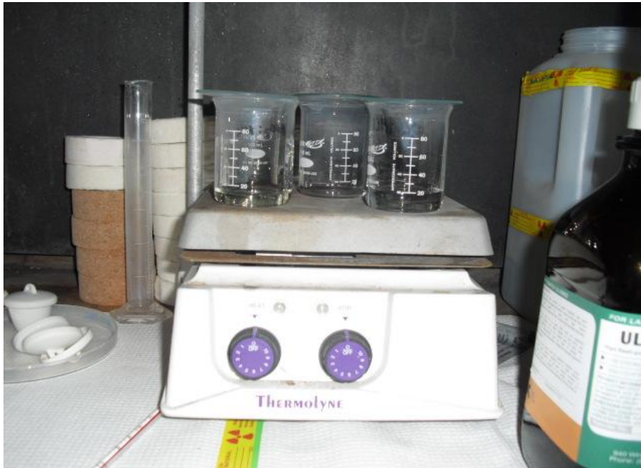
Figure 2.4. Wet oxidation process, showing aqueous fish sample in beaker
