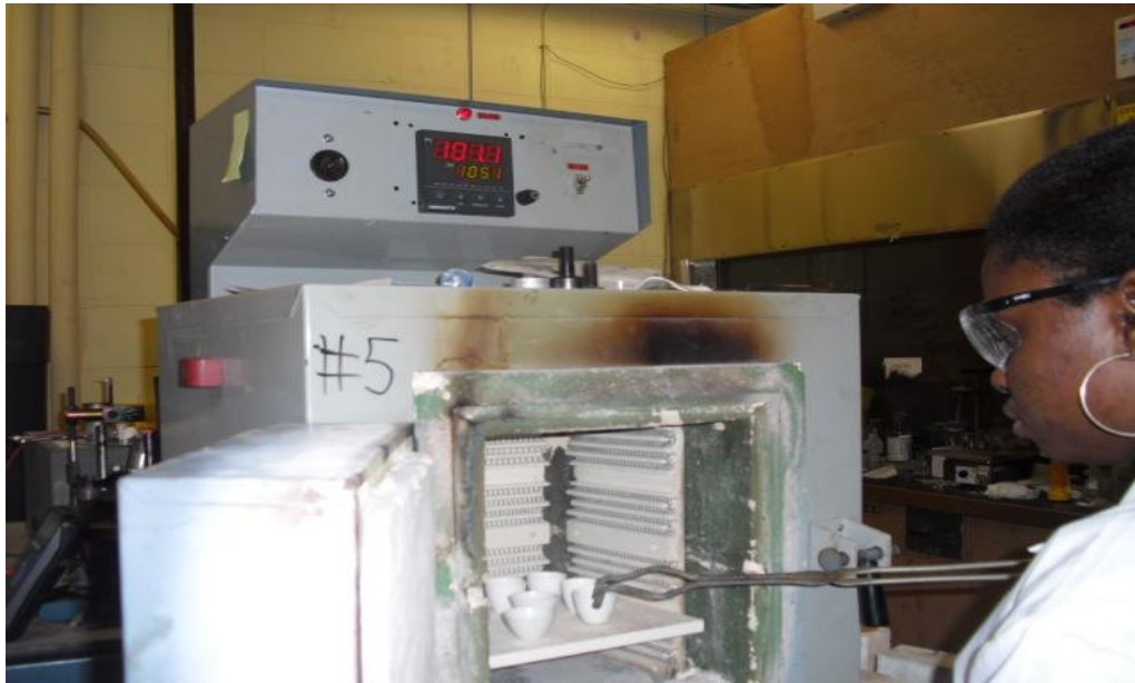
Figure 2.3. Calcination of fish whole body
