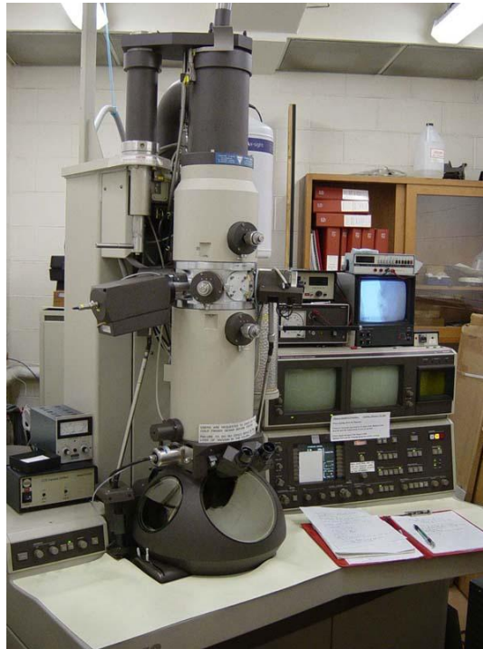
Figure 3.7: Philips CM12 conventional analytic TEM operating at 120kV
