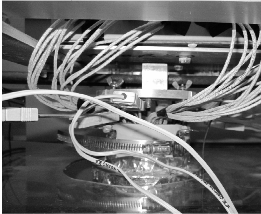
Figure 2.8: Fully Instrumented Heated Element, Confined Variation
