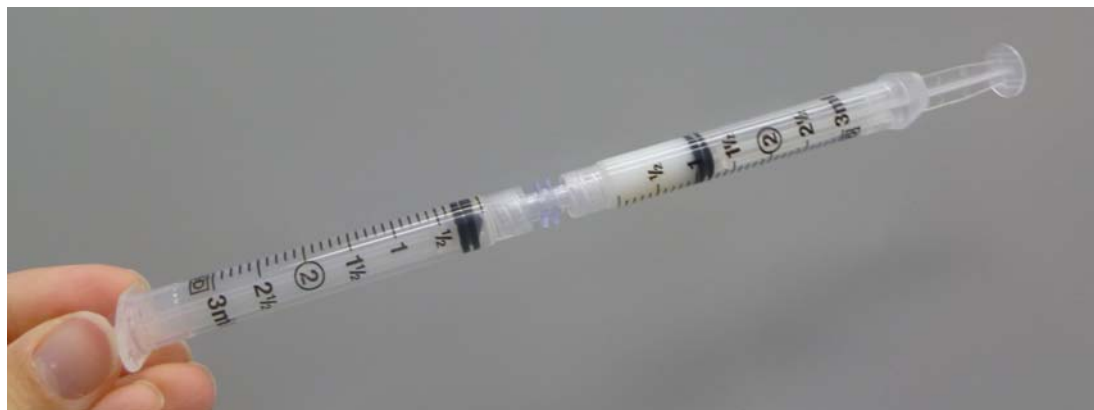
Figure 9-1. Syringe mixing system for collagen gel formation.
