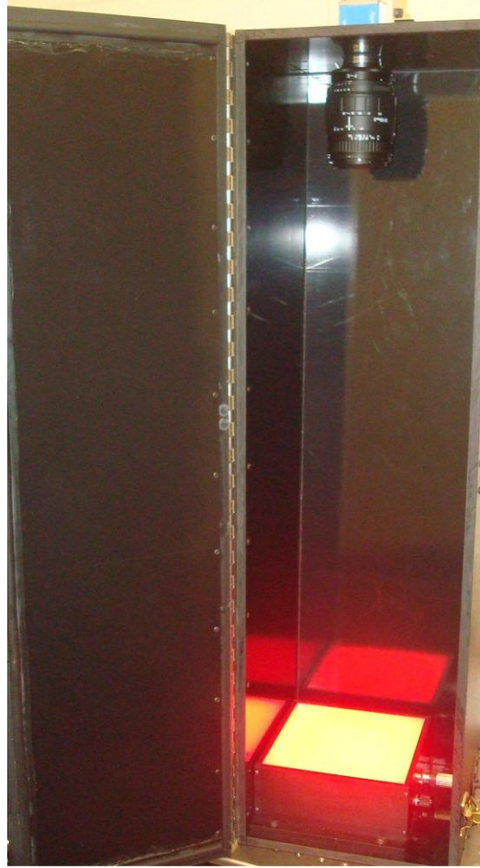
Figure 2.7 Picture of in-house 2D optical scanner, a red light surface in a light tight box with a lens-coupled CCD on top.
