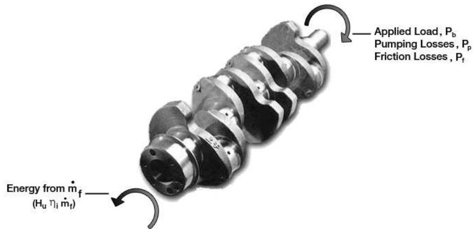
Figure 3-6: Physical depiction of crankshaft equation. Fuel flow into the cylinders is modified by the fuel heating value and engine thermal efficiency to give the energy input. This is then balanced against the load and losses to yield the state equation.
