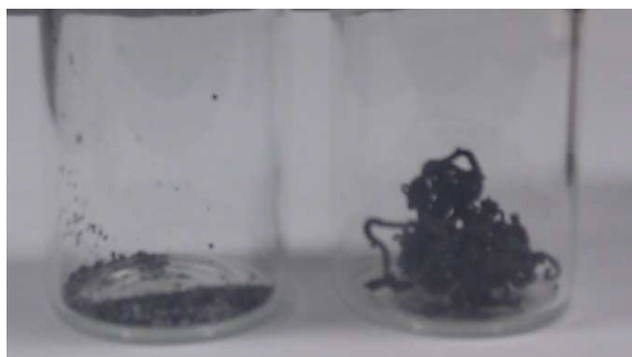
Figure 4.2: Image of expandable graphite (left) and expanded graphite (right) after expansion in the vacuum evaporator at 4 amps.
