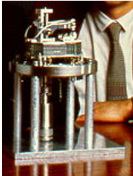
Figure 2.1: The first scanning tunneling microscope invented by Gerd Binnig and Heinrich Rohrer.
