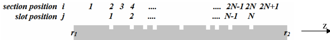
Figure 6.2 1D approximation of the DM laser along the longitudinal direction.
