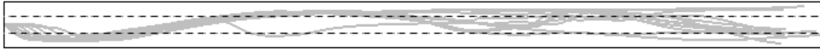
Figure 4.24: Particle tracks for Re = 718 . Image is looking down on the domain, flow from left to right. Dashed black lines indicate location of the rod. Tracks are shown for particles over a time span of 2.25 seconds, starting at 70 seconds into the true transient. The particle tracks were set to stop once the particles had travelled about 750 mm.
