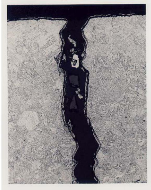
**Figure 5.1- Quench crack in forged AISI 403 martensitic stainless steel [30]**
