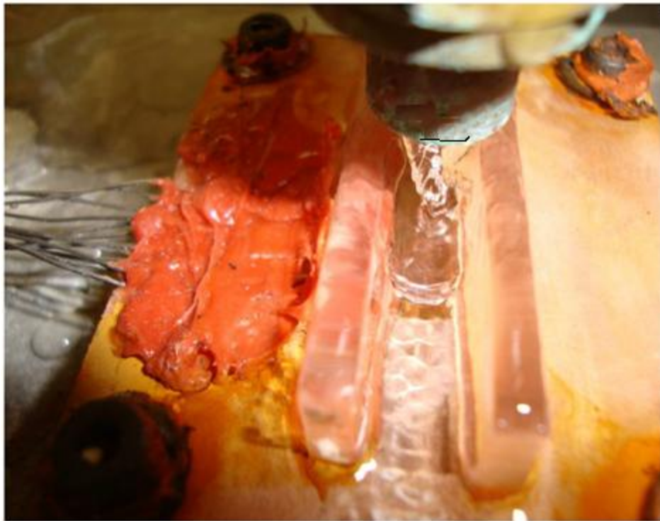
Figure 4-3 Photograph of the Flow Field taken at Jet Velocity of 1.5 m/s
