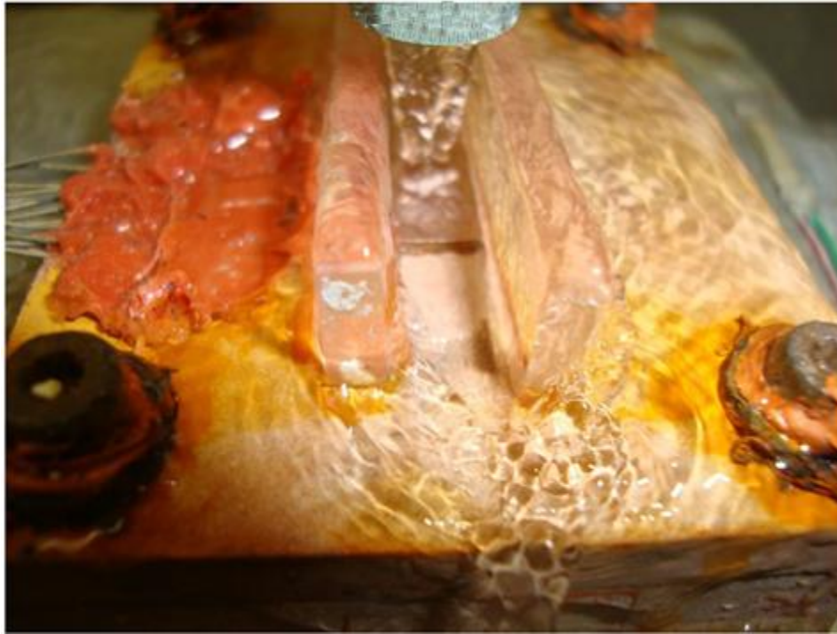
Figure 4-4 photograph for the flow field taken at jet velocity of 2.5 m/s
