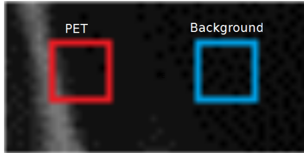
Figure 3.5: Enlarged Boundary Region of a PET Bottle. The red box contains similar pixels to the blue box, the only difference is the presence of the specular reflection
