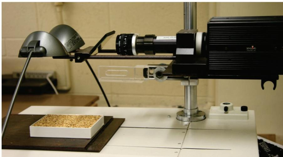
Figure 4.1 Desktop line-scan NIR imaging spectrometer
