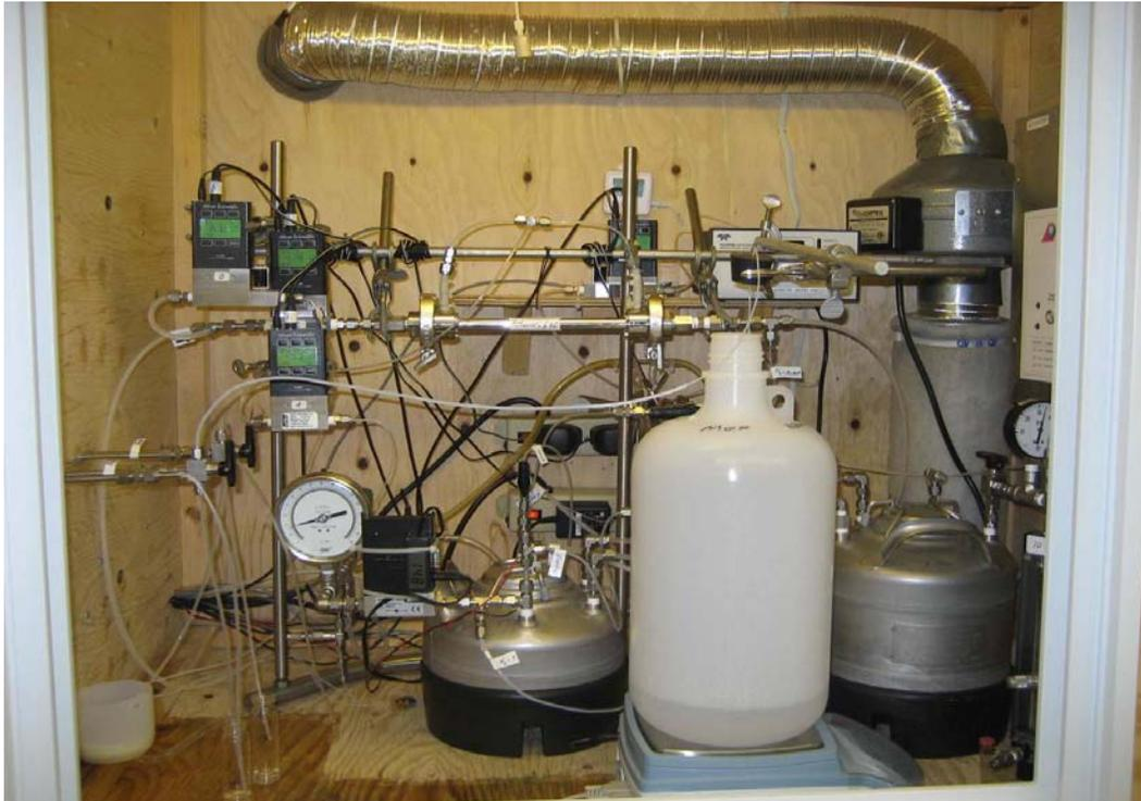
Fig. A1- Experimental apparatus: Hybrid ozonation – membrane filtration.
