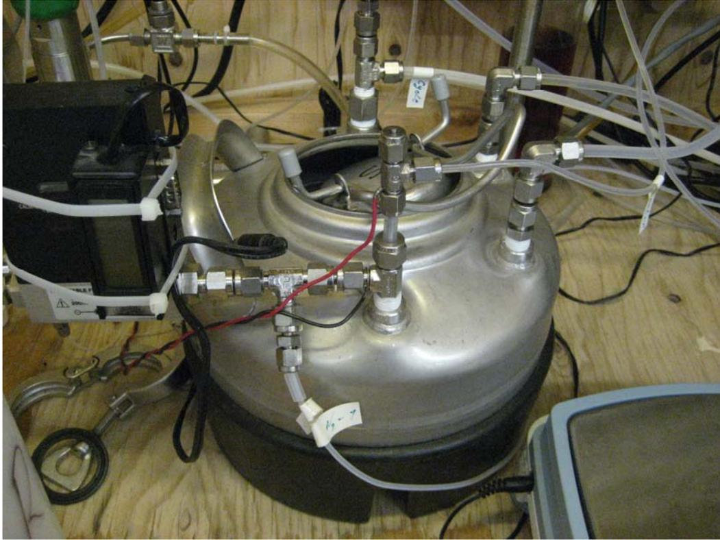
Fig. A2- High-pressure stainless steel tank.
