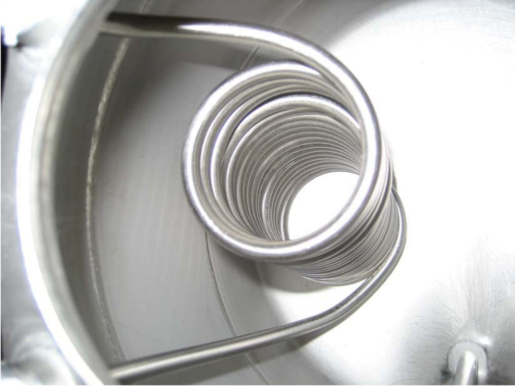
Fig. A3- Water coil inside the tank.
