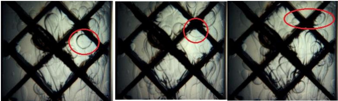
Figure 28. Image sequence showing drop breakup from impact with cross-points of the packing
