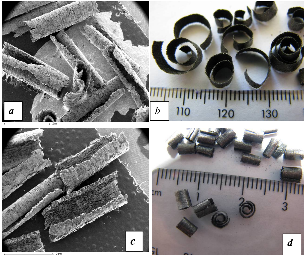
Figure 53 CGI segmental chip at different feed rate and cutting speeds 0.05 mm/rev @ 200 m/min (a), 0.1 mm/rev. @ 200 m/min (b), 0.2 mm/rev. @ 200 m/min (c), 0.1 mm/rev @ 400 m/min (d).
