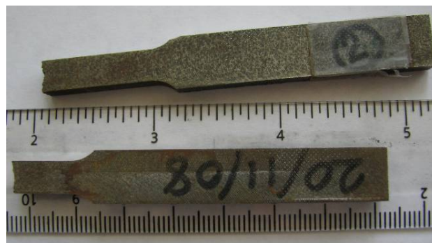
Figure 25 Tensile test specimen ASTM E8
