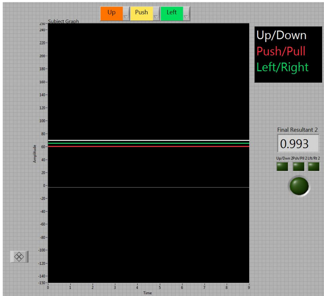
Figure 3.2: Screen capture of the visual display viewed by subjects during their exertions. An example of an up/push/left 3D exertion is shown, where the goal of the subjects was to match the 3 horizontal lines (equal force on all three axes) at their maximal force level. The white line represented the up/down force, the red line represented the push/pull force and the green line represented the left/right force.
