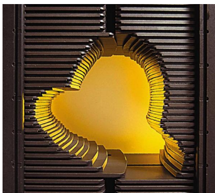
Figure 1.1: A multi leaf collimator (MLC) producing an intensity-modulated field with moving the leaves when the beam is on and perpendicular to this page (Bortfeld, 2006).
