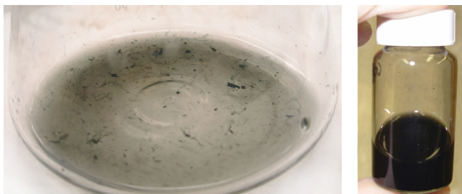
Figure 31 – [Left] A photo of a functionalized nanotube solution poured into a wide flask after much of the material had precipitated into visible fiber-like particles. [Right] A photo of the original functionalized nanotube solution as received.
