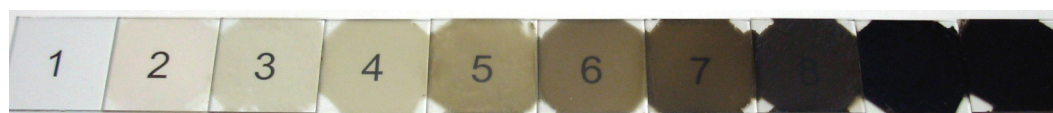
Figure 54 - A photograph of a series of polymer functionalized SWNT coatings deposited on ITO. They are arranged in order of increasing coating thickness and placed over printed numbers to help visualize the transparency of each coating. The first specimen is uncoated for comparison.
