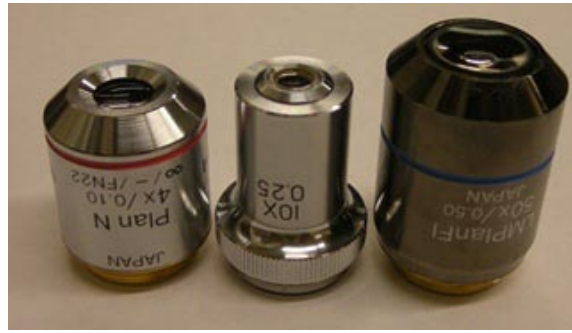
Figure 5.15: Different microscope objective lens, from left to right 4x/0.10, 10x/0.25, 50x/0.50.
