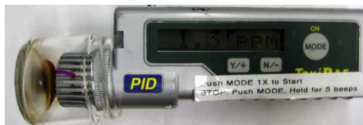
Figure S4. ToxiRAE Plus PID gas detector is connected to a 40 mL glass bottle where 700 \mu L of reaction mixture produces methyl mercaptan.
