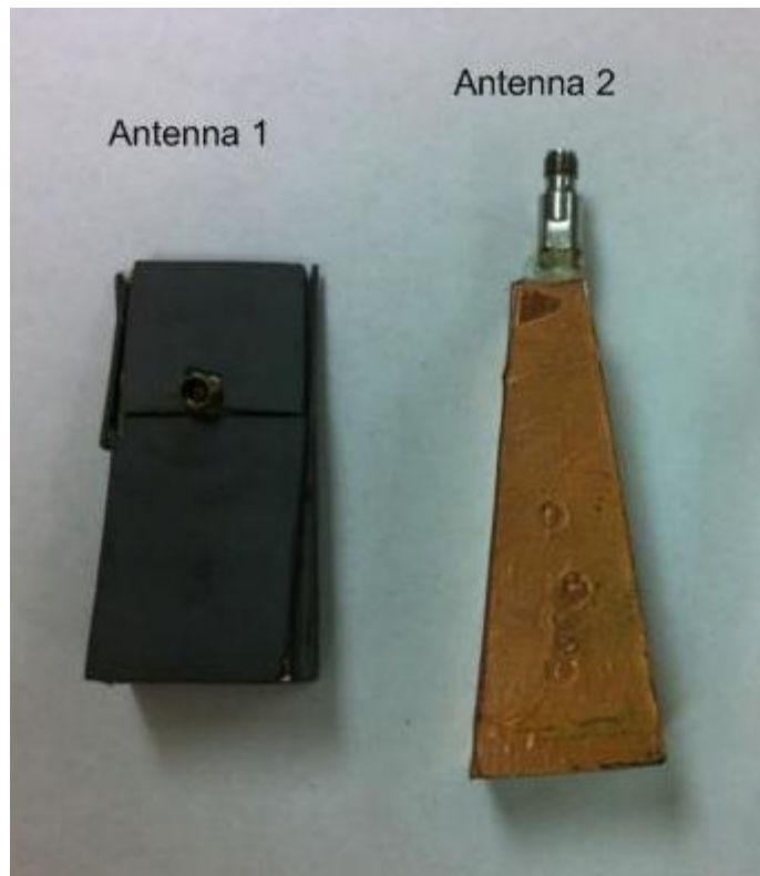
Fig. 4.1. Photo of the two imaging antennas used in the raster-scanning setup.
