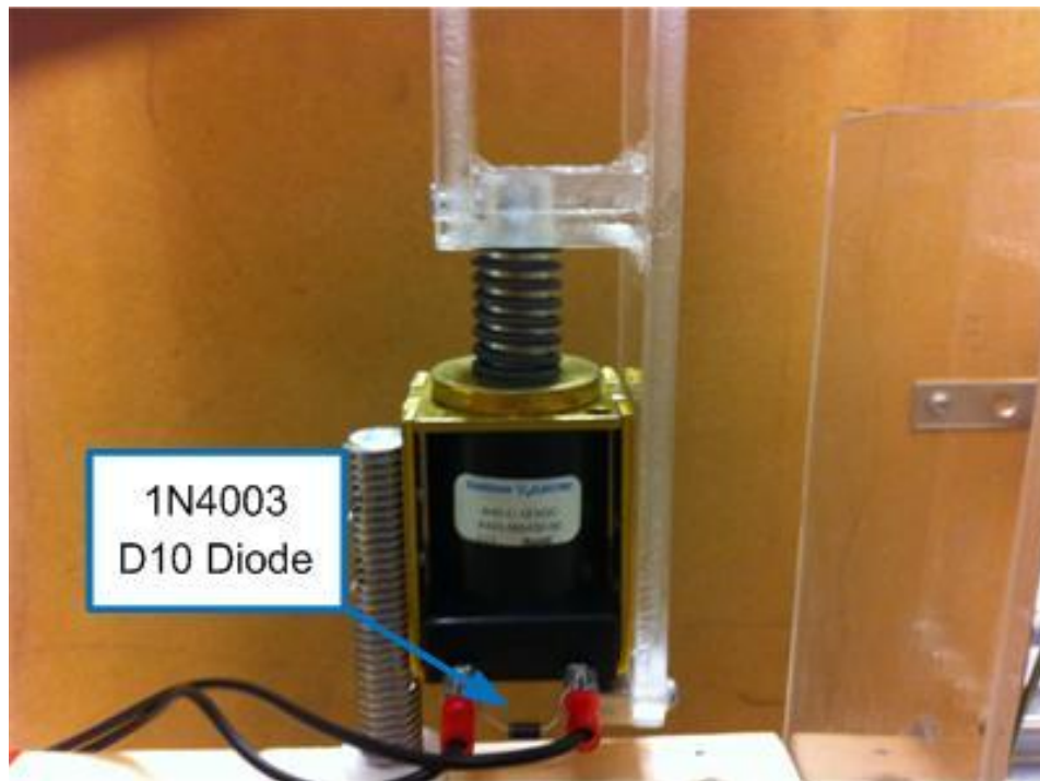
Fig. 2.19. Connections of the bottom solenoid.
