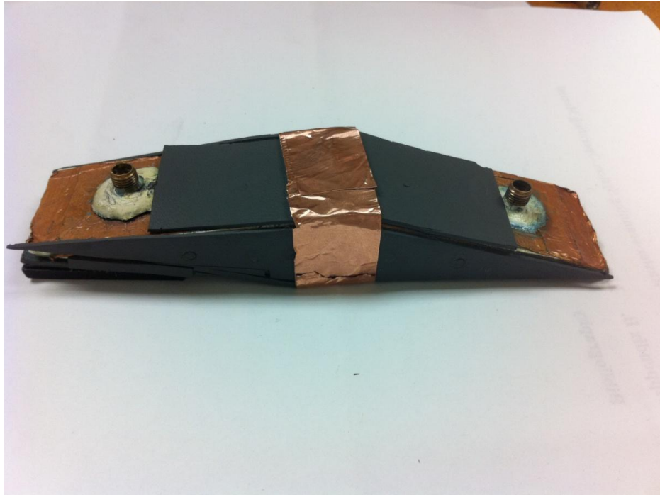
Fig. 4.4. Configuration with antenna 1 for measuring the maximum coupling efficiency.
