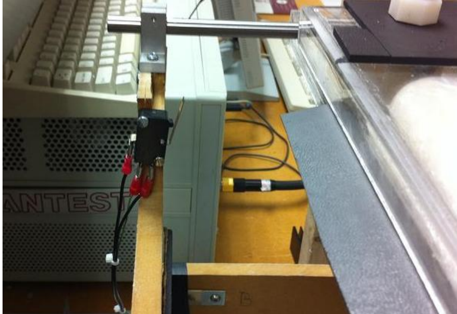
Fig. 2.23. Close-up of switch 3 at top of the scanning table frame.
