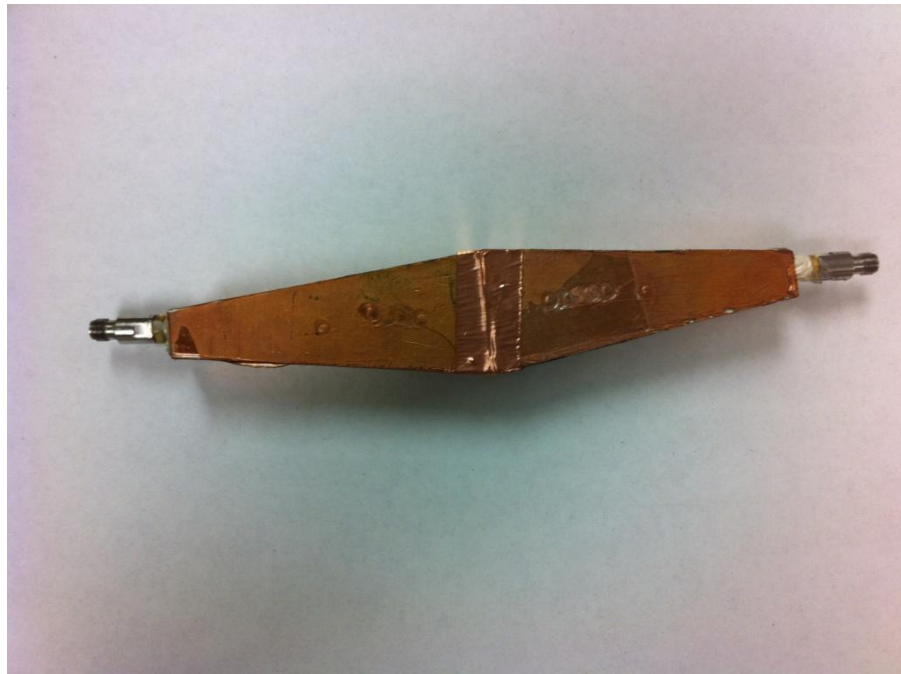
Fig. 4.5. Configuration with antenna 2 for measuring the maximum coupling efficiency.
