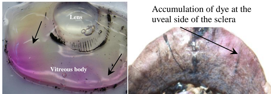
Figure 32. Delivery in ex-vivo bovine eye: intravitreal delivery (A) of dye and (B) dye penetration in the posterior segment after release from the microneedle array
