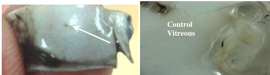
Figure 64. Microneedle insertion point (shown by arrow) is visible on the uveal side indicating microneedle penetration through the sclera. However, there was no observable evidence of any dye released to the vitreous humour through passive diffusion alone.
