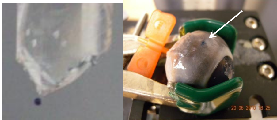
Figure 52. A 126 \mu\text{m} microneedle showing a droplet of trypan blue from a 126 \mu\text{m} OD/10 \mu\text{m} ID; the insertion point (white arrow) is visible after the device was removed
