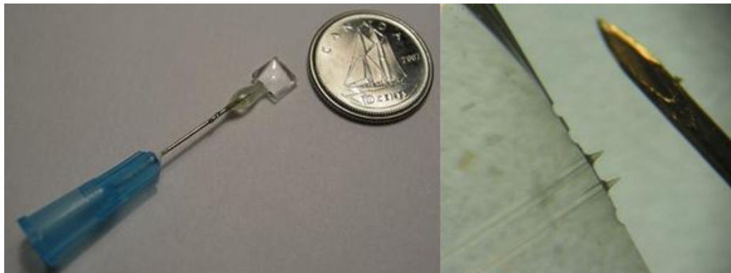
Figure 85. Size comparison of 2 X 126 \mu\text{m} OD/10 \mu\text{m} ID microneedles embedded into micropatterned PDMS substrates. Microneedles are shown next to a 30 Gauge stainless steel needle (305 \mu\text{m} OD X 140 \mu\text{m} ID) currently used for intravitreal injections
