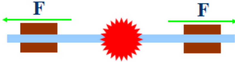
Figure 9. Schematic showing micropipette fabrication: a single borosilicate capillary tube is pulled biaxially while heating the midpoint to 585°C to form two micropipettes with taper lengths of 9 mm and tip diameters in the range of several microns.
