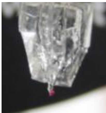
Figure 54. Droplet of rhodamine emerging from the tip of a 1.1 mm tall 323 \mu\text{m} OD/10 \mu\text{m} ID microneedle
