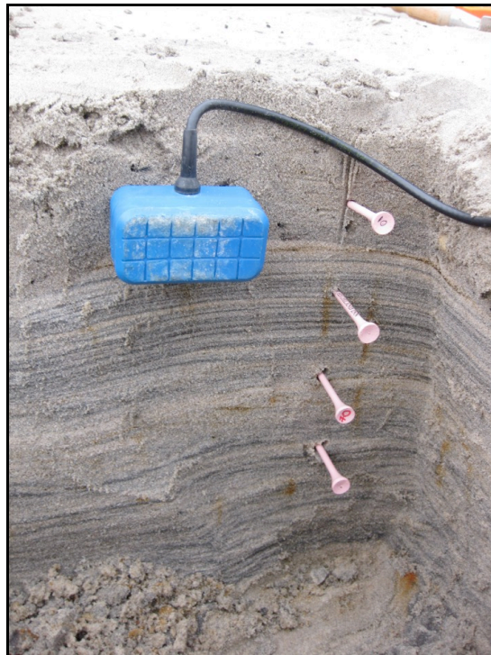
Figure 3.6: Collection of in situ volumetric moisture contents within sampling pit (top) and close-up of Time Domain Reflectometry (TDR) probe used (bottom), August 2009.
