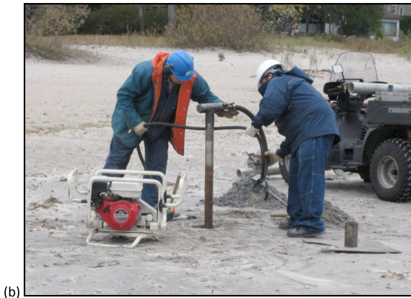
Figure 3.7: (a) Diagram of the vibra-corer, (b) example of vibracoring to obtain particle samples in the saturated zone, October 2009.
