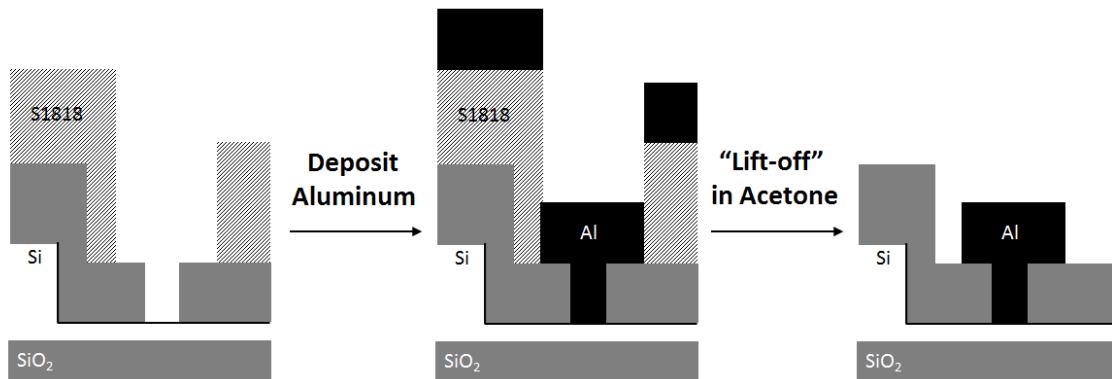
Figure 5.9: ‘Lift-off’ process of forming patterned Aluminum contact on doped region adjacent to waveguide edge (half of the waveguide cross-section is shown here for illustration): Photoresist development of pattern (left), aluminum deposition (middle), and ‘lift-off’ of photoresist and Aluminum coating in warm acetone (right).
