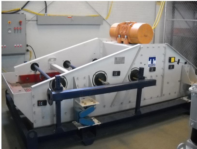
Figure 11.1: Linear Vibrating Screen - Side View
