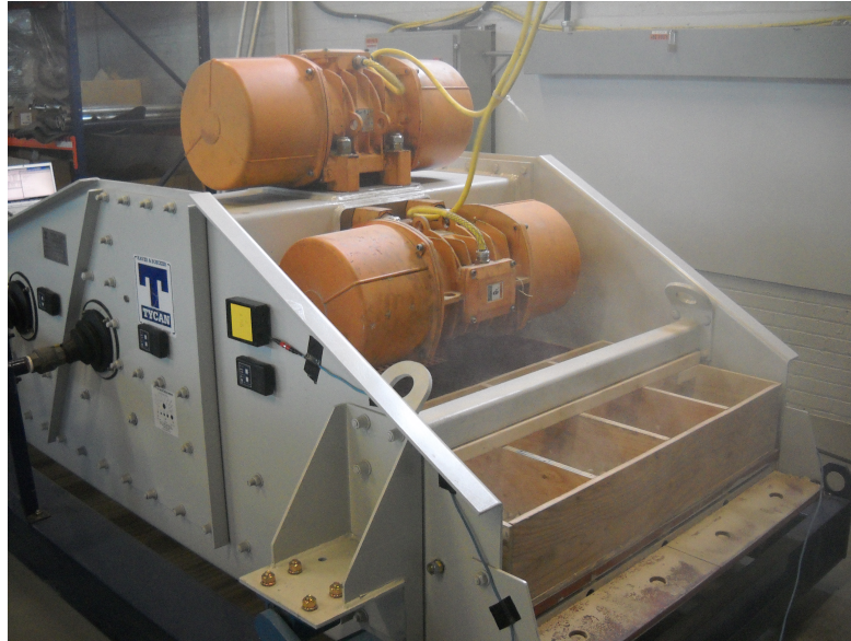
Figure 11.2: Linear Vibrating Screen - Discharge End View
