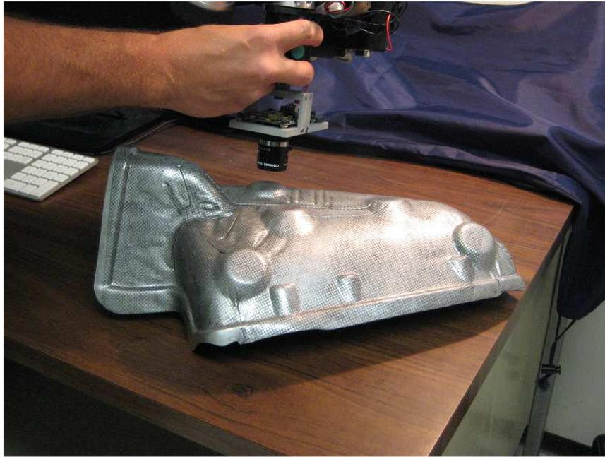
Figure 2.16: Scanning automotive heat shield surface using single camera mounted to FARO arm.
