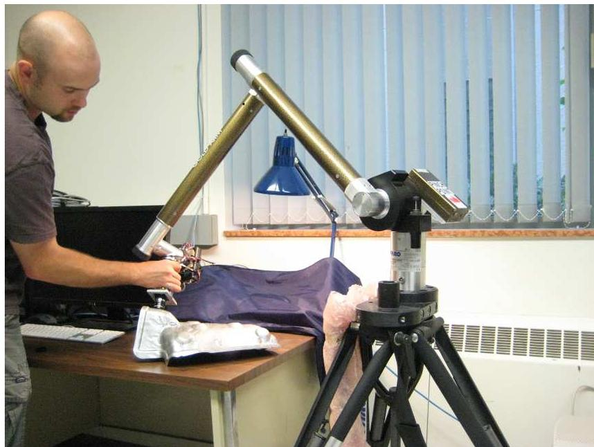
Figure 2.15: Scanning automotive heat shield surface using single camera mounted to FARO arm.
