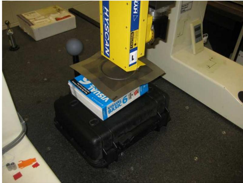
Figure 1.2: Gantry CMM-mounted laser scanner measuring surface geometry of metal dome.
