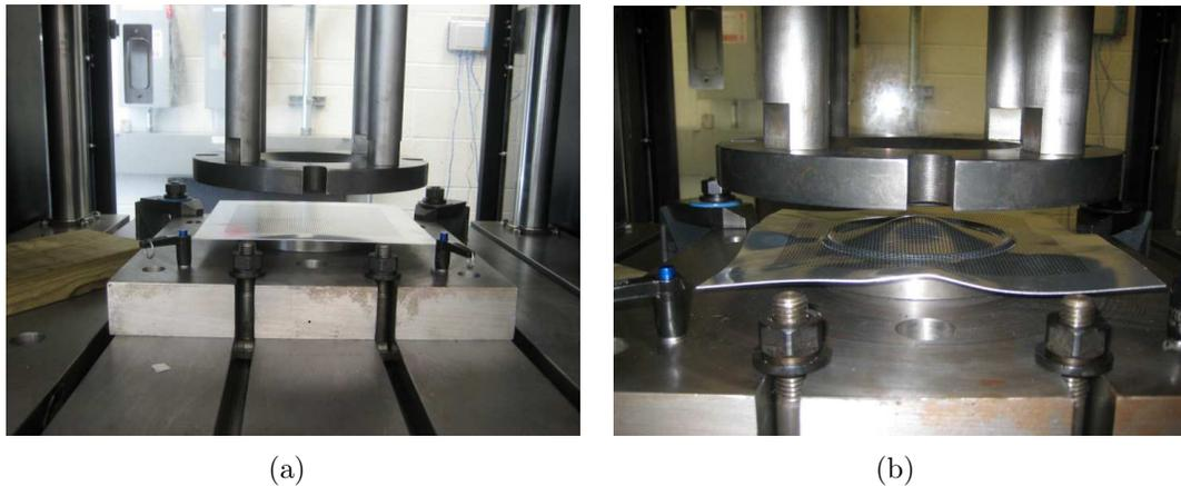
Figure 1.1: (a) Flat sheet metal sample before deformation; (b) Sheet metal sample deformed into a dome to measure material properties.
