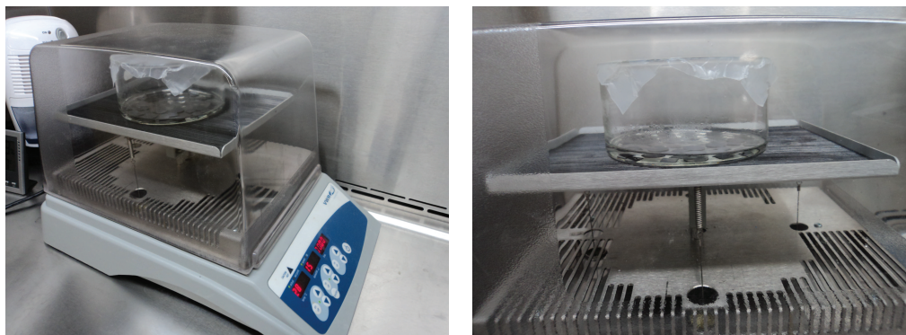
Figure 3.9: The VWR tilting incubator is shown here with wafers in APTES. The rate and angle of tilt can be controlled, as well as the temperature inside the enclosure.
